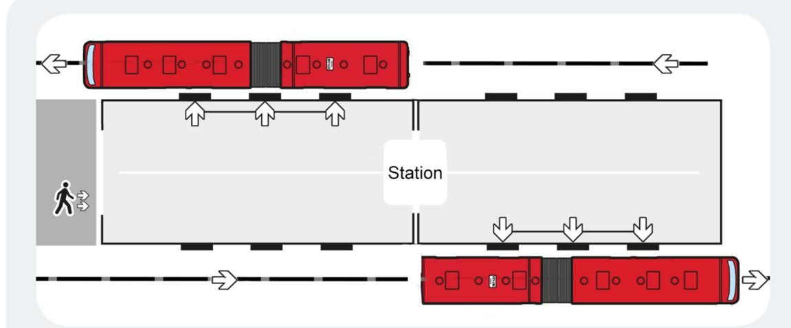
Left: A typical bus station layout, as it exists in many (not only) Latin-American countries. The Trans Milenio System, nevertheless, partly consists of more complex bus stations (right). The stations include two sub-stations, can be accessed by two-plus-two busses and two lanes per direction. On each bus berth various bus lines can halt.
